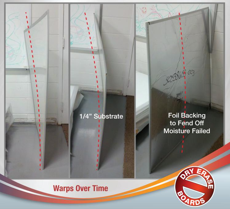
These actual unedited photos show two different dry erase boards that, after a short time, have taken on a shape of their own. Very different condition from when originally purchased. These are high-end, porcelain-on-steel construction made by a MAJOR brand name. The first board is constructed using a 1/4" substrate, the second using a 1/2" substrate, both with particle board. The condition of these boards are the most undesirable result possible for use with a projection system.
